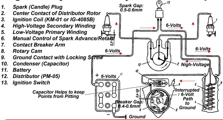
The basic ignition system is simple. The breaker points are normally closed, allowing the magnetic field to build in the ignition coil. When the cam shaft rises, opening the breaker points, the collapsing magnetic field induces a high-voltage in the secondary winding of the coil.
