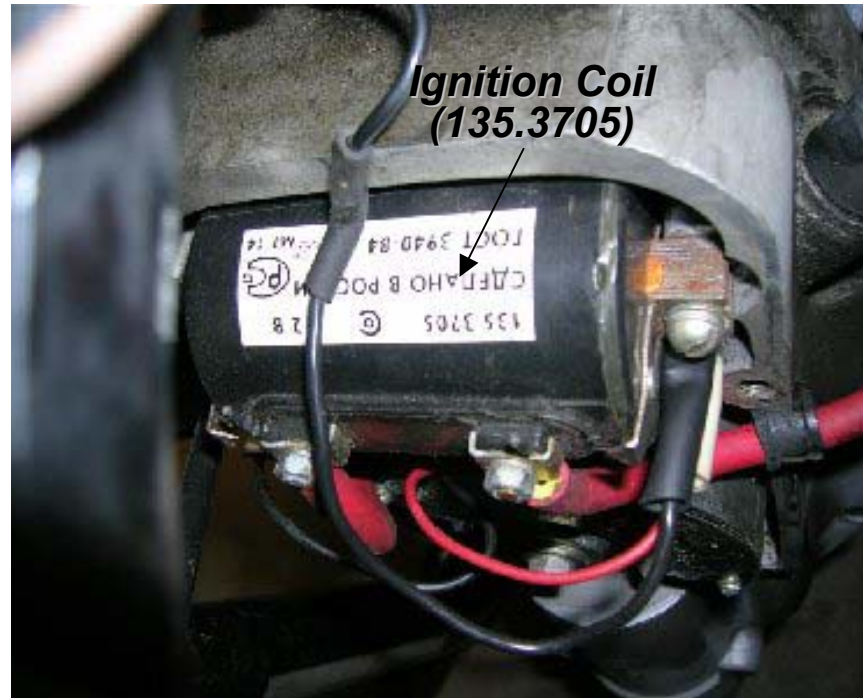
Upper View of Front Ignition Compartment Showing Ignition Coil
