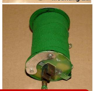
The B201 became the standard ignition coil for 6-Volt Urals and Dneprs.
