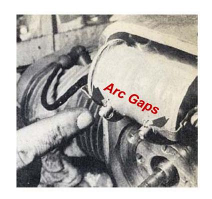
The ignition coil is double-ended with two spark safety gaps, which were set at 9 mm (0.355").
