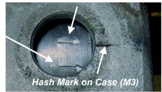
750cc Urals have two marks on the flywheel; TDC and the timing mark. The arrows come into view on the compression stroke. The TDC mark is the arrow WITHOUT the dot at the shaft (-->), while the arrow shaft WITH the dot (0-->) is used to set ignition timing.
